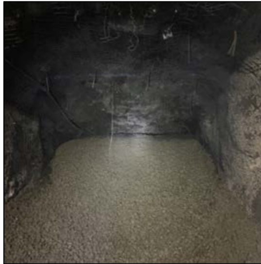
Jam Backfill in the 381-1425 Secondary Sill
